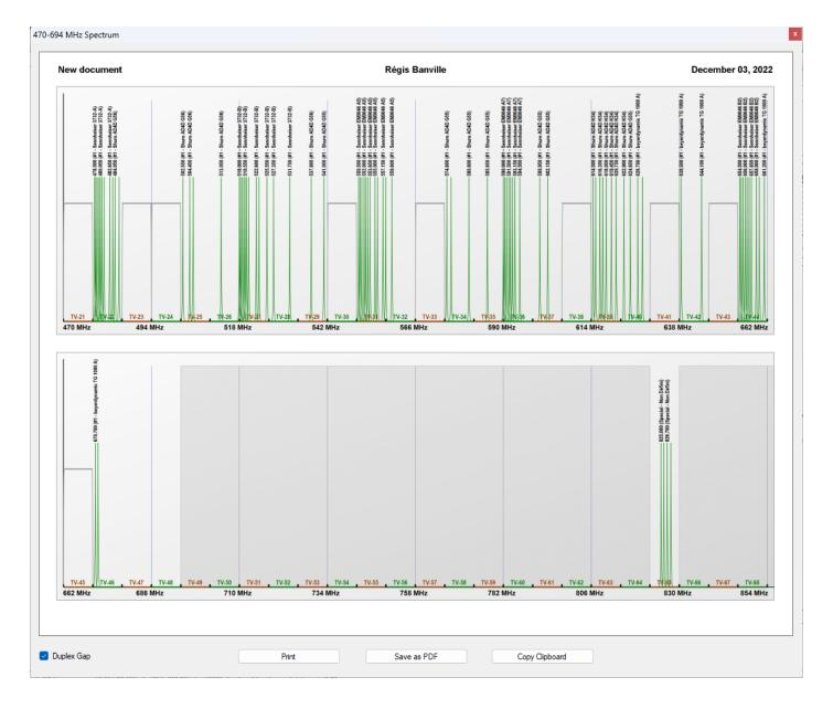
The purpose of the module is to illustrate the entire RF space by spreading the frequency range over two sections in order to be able to print it on a single page or do the viewing without moving.
