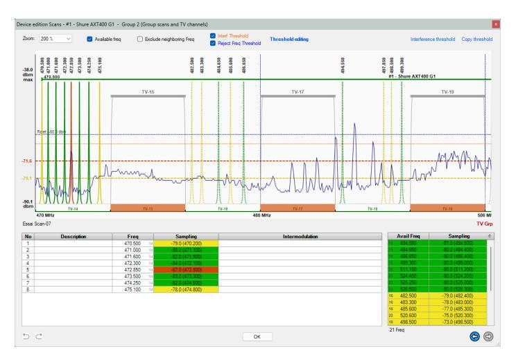
The frequency analysis is based on the level of the samples, the value of the rejection width of the interference frequencies (0.300 MHz by default) is used for the calculation (document parameters).
