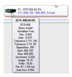
The last parameter displayed, Auto-Increment, is a parameter calculated by EazyRF to accelerate calculations. Thus, when the increment is larger, the number of frequencies tested decreases. The value of this parameter depends on several factors, the main ones being Tolerance 2 and 3 TX.
